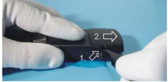
To remove the Battery Cover push the lock button with plastic tweezers and then push the Battery Cover forward softly.
