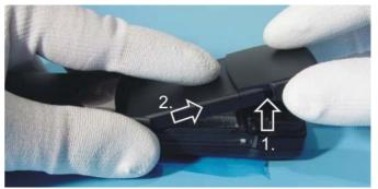
Lift the Battery Cover up and then pull it out carefully.
